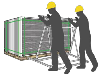
3) Place the stand supporter that is higher or wider than the module in order to avoid hitting and damaging the glass.
